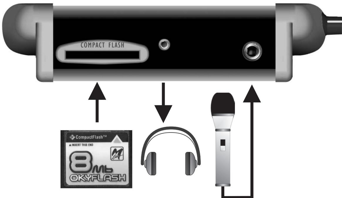
**MIC IN**                      Microphone connection socket.
