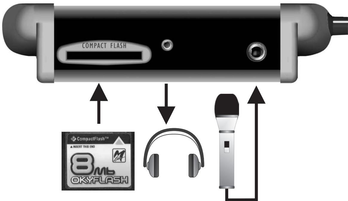
**MIC IN**                      Microphone connection socket.
